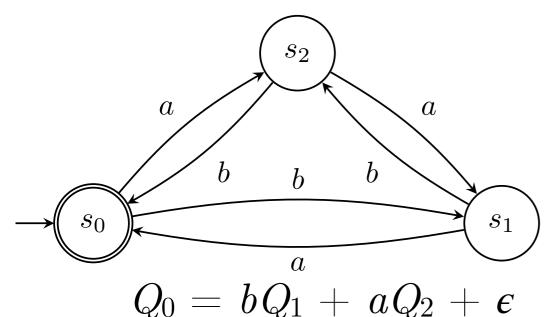
$$egin{aligned} Q_0 &= \, b \, Q_1 \, + \, a \, Q_2 \, + \, \epsilon \ Q_1 &= \, a \, Q_0 \, + \, b \, Q_2 \ Q_2 &= \, b \, Q_0 \, + \, a \, Q_1 \end{aligned}$$
