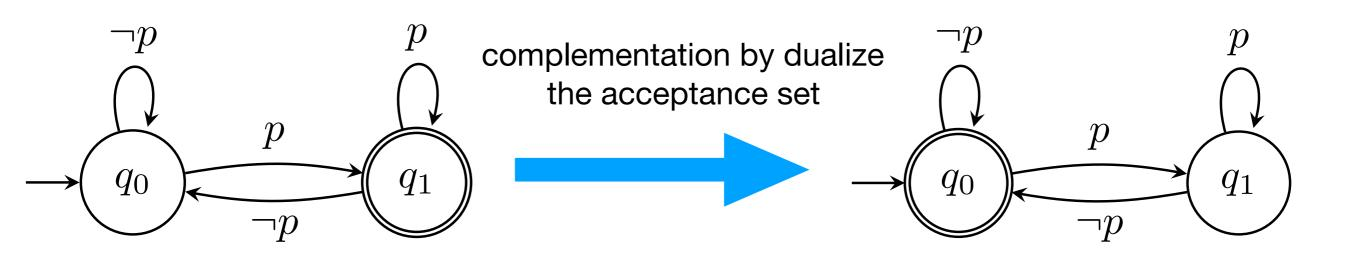
Does the right one exactly accept the complement of the left one Complementation of NBW is much harder than that of NFA.
