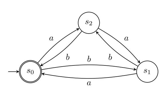
$$egin{aligned} Q_0 &= \, b \, Q_1 \, + \, a \, Q_2 \, + \, \epsilon \ & \ Q_1 &= \, a \, Q_0 \, + \, b \, Q_2 \ & \ Q_2 &= \, b \, Q_0 \, + \, a \, Q_1 \end{aligned}$$
