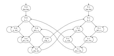
The value of the outer program counter is not shown. Initially, the program counters of both processes have the value bot  $(\perp)$ , indicating that they are not started yet.
