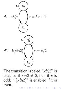
Automata-Based Model Checking
